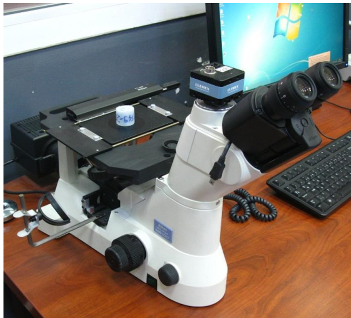
Figure 4.4 : Nikon Eclipse MA 100 with Clemex Image Analyses System
