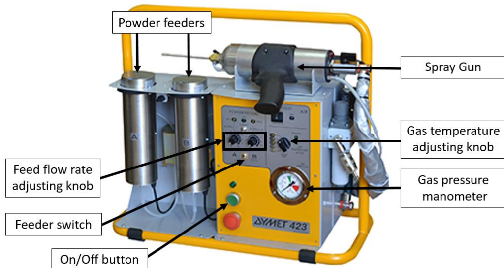
Figure 4.1 : Dymet 423 LPCS equipment
