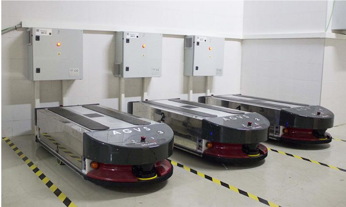
Figure 1.15: AGVS: Mobile Platforms for Intrahospital Logistics [16]
