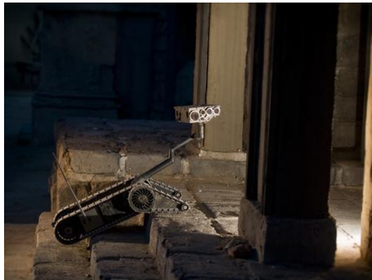
Figure 1.18: XM1216 Small Unmanned Ground Vehicle (SUGV) [19]
