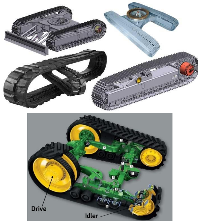
Figure 1.8: Line Type Tracked System [9]
