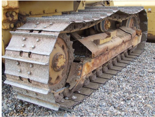
Figure 2.9: Closeup of Geared Tracks on a bulldozer [57]
