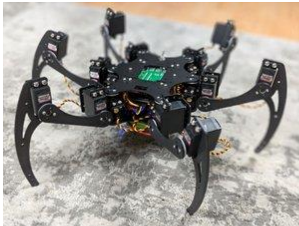
Figure 1.6: Capers II, a Hexapod Robot [7]
