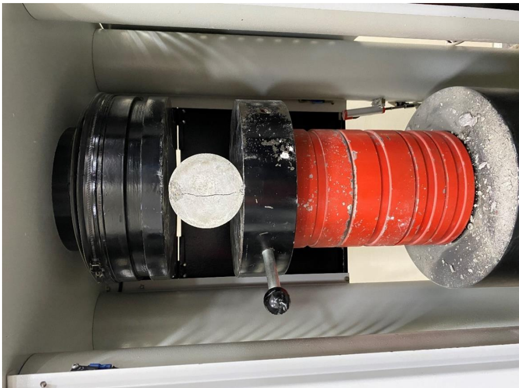
Figure C.6 Split tensile test of cylinder concrete sample having 100 mm diameter and 200 mm height
