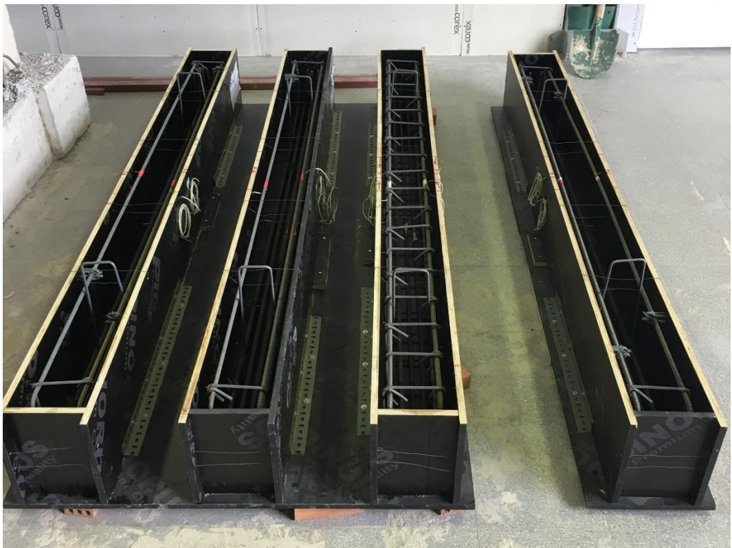
Figure C.2 Reinforcements placed into the prismatic molds, before concrete pouring
