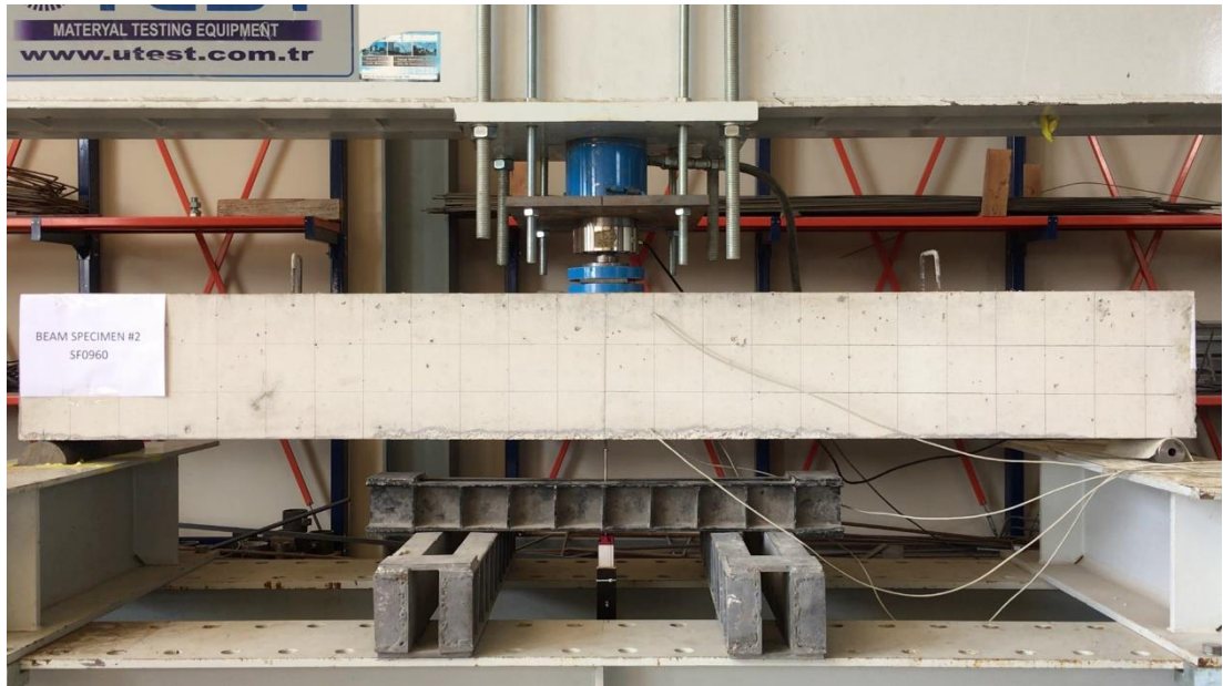
Figure 4.1: Beam specimen and the sensors ready for test
