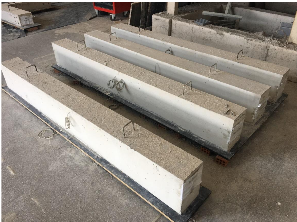
Figure C.4 The beam specimens after removing the formworks and ready for testing
