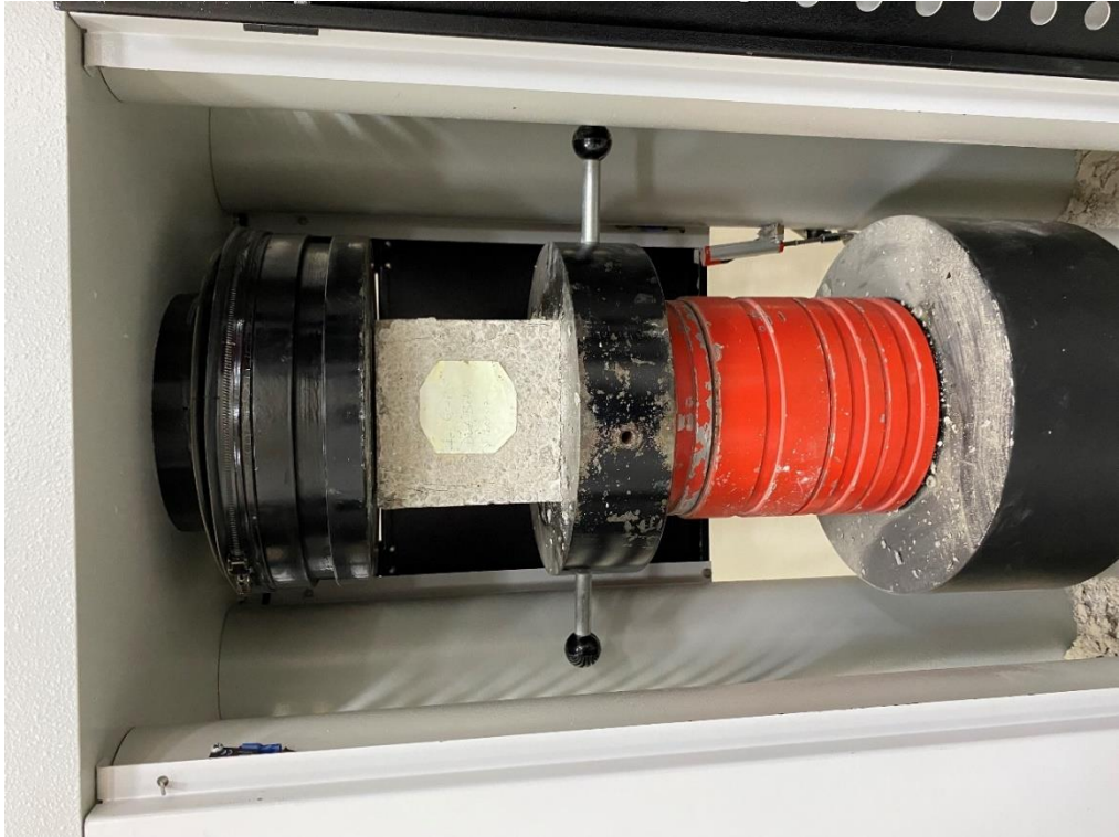
Figure C.5 Compression test of 150 mm x 150 mm x 150 mm standard cube sample
