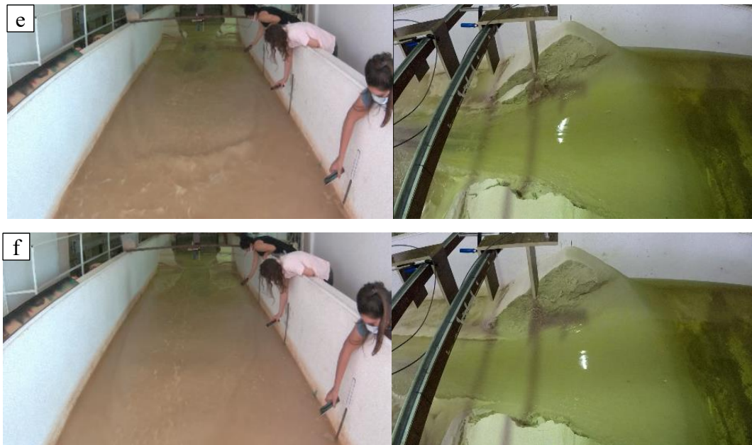
Figure 4.2 : Camera 2 (flow and sediment transport at downstream area) and Camera 1 (stages of breach formation) at a) 282 s, b) 307 s, c) 322 s, d) 342 s, e) 357 s, f) 387 s for experiment OS1
