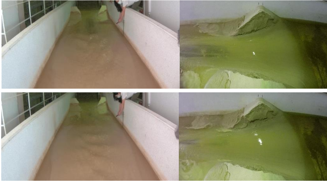
Figure A.A.1: Camera 2 (flow and sediment transport at downstream area) and Camera 1 (stages of breach formation) at a) 291 sec, b) 311 sec, c) 331 sec, d) 351 sec, e) 361 sec, d) 375 sec for experiment OS2
