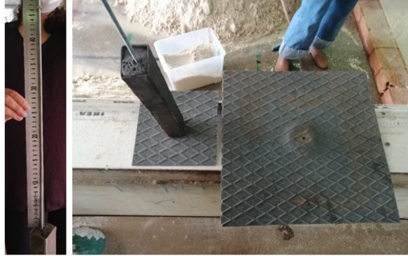
Figure 3. 6: Compaction materials; iron weight and plate
