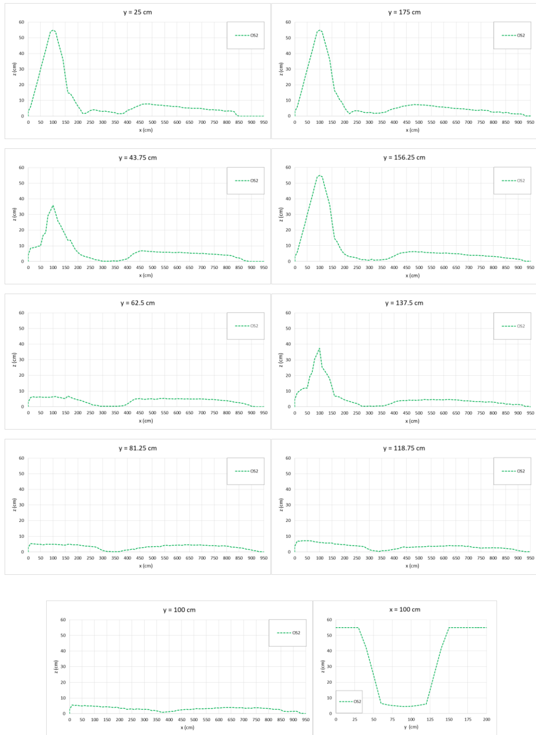
Figure A.A.5: Longitudinal sediment height profiles measured at a) y = 0 cm and 200 cm, b) y = 12.5 cm and 187.5 cm, c) y = 25 cm and 125 cm, d) y = 43.75 cm and 156.25 cm, e) y = 62.5 cm and 137.5 cm, f) y = 81.25 cm and 118.75 cm, and g) y = 100 cm and along the channel width and, transversal crest section of the dam at h) x = 100 cm of OS2
