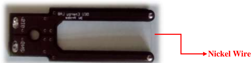
Figure 3.7 : Thermal probe operating both as heater and thermometer.
