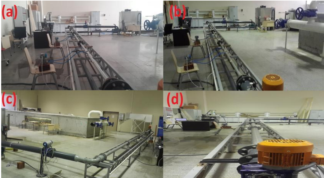
Figure 3.2 Izmir Katip Celebi University Civil Engineering (IKCU-CE) Flow Loop and galvanized pipes with different diameters (a. 40 mm, b. 50 mm, c. 80 mm, d. 90 mm)
